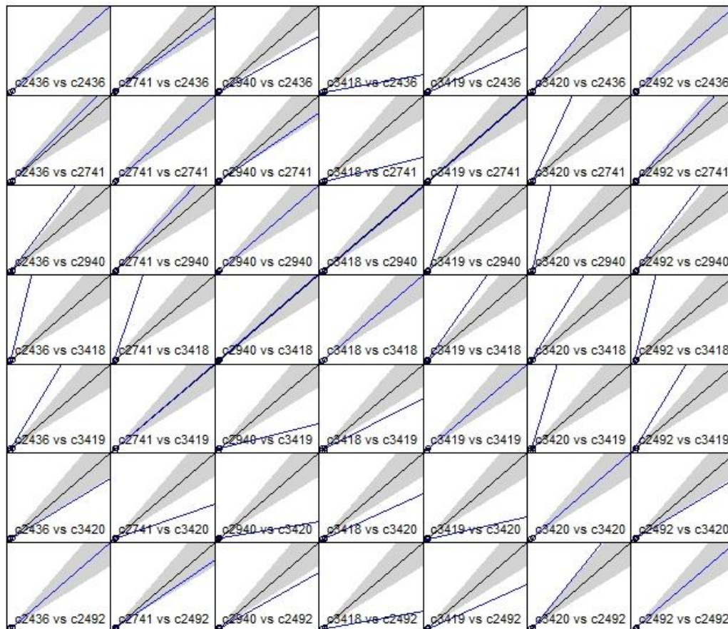
Figure 4.1: Orthogonal regression plot of C-POD comparisons in calibration trial (June-July 2019), in blue, with a null model where each unit performs exactly the same, in black and an acceptable error margin of \pm 20\% , in grey from Calibration trials, June-July 2019.
