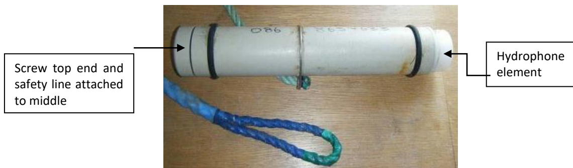
Figure 3.2: C-POD unit by Chelonia Ltd
